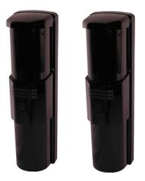
The DS484Q and DS486Q Detectors have separate transmitters and receivers. The transmitter sends an invisible infrared beam to the receiver. If the beam is broken, the receiver signals an alarm. Multiple channel operation provides increased system flexibility.
